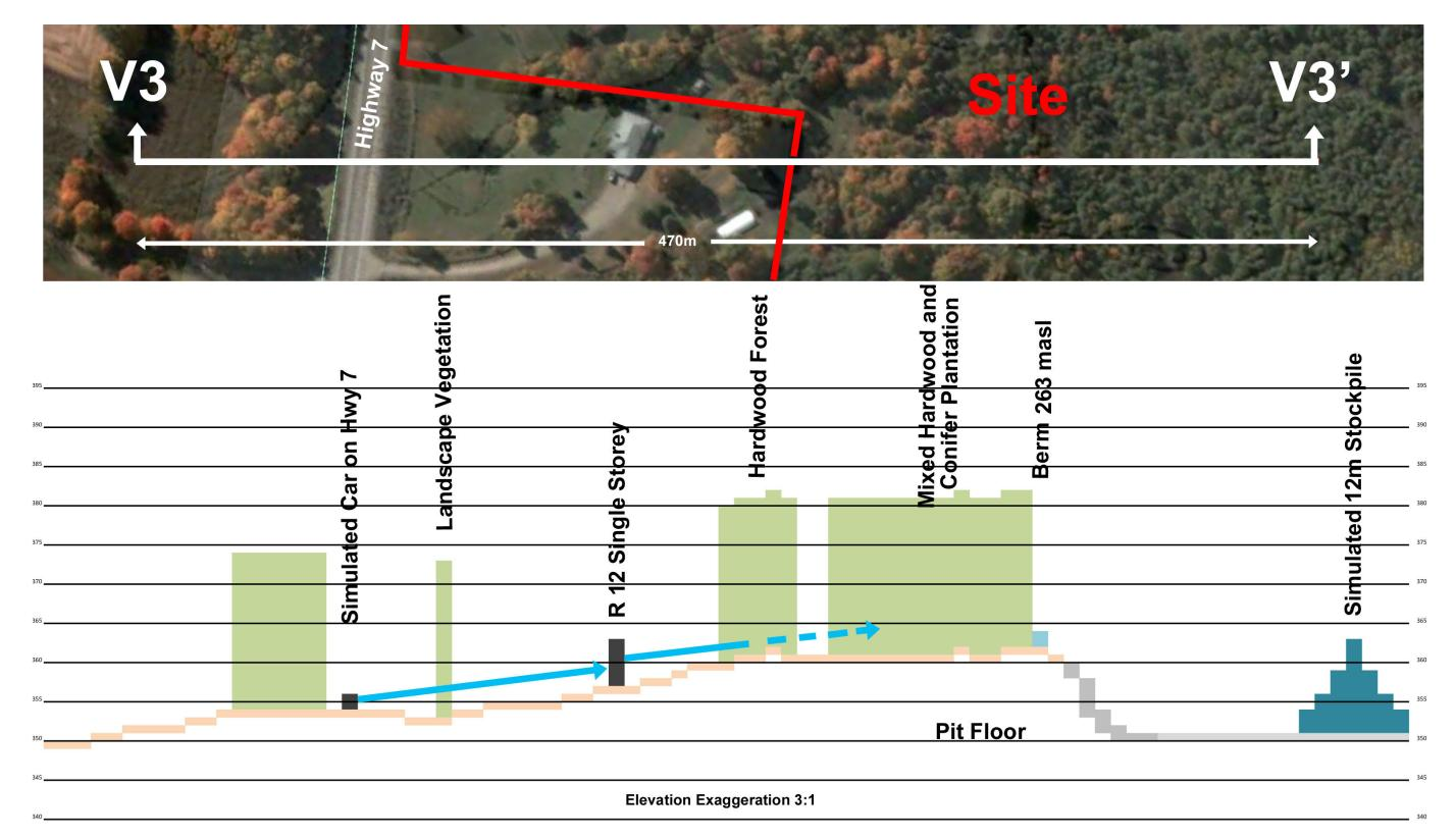
Figure 13- Cross Section V3-V3' Analysis- Quarry not visible from any receptor. Heavy existing tree cover in existing bush and large setbacks completely hide quarry. See Photo 5.
