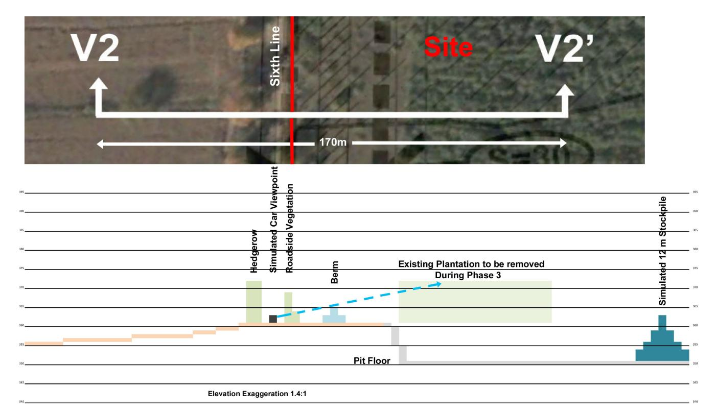
Figure 12- Cross Section V2-V2' Analysis- The quarry is not visible. The berm is visible through gaps in the roadside vegetation screen. The berm itself is to be reforested. See photos 12 and 13. The coniferous plantation is not to be removed until Phase 3 (approximately year 12 of the operation), at which time the reforestation on the berm will have achieved some size.
