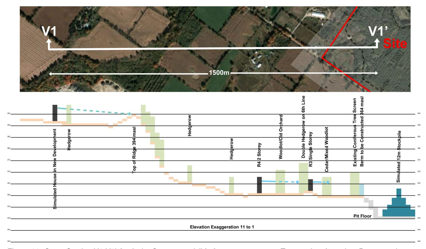
Figure 11- Cross Section V1-V1' Analysis- Quarry not visible from any receptors. Trees to be planted on Berm not shown.
